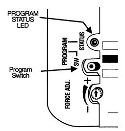
At this point you will be able to activate the opener. It will open, but will not close the door. Before unit will close door the beam sensors must be aligned and programmed (next step).
